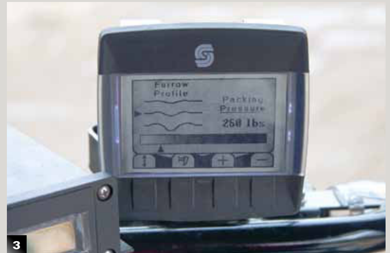
[1, 2] Independent shank with mechanical linkage [3] In-cab monitor with seed furrow selection
