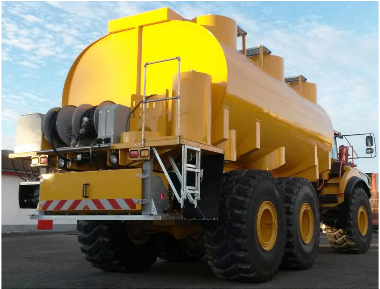
Coolant tank (right side) with electrically / pneumatically driven pump Spring loaded hose-reel, 15 m hose and integrated flow-meter in discharge nozzle
