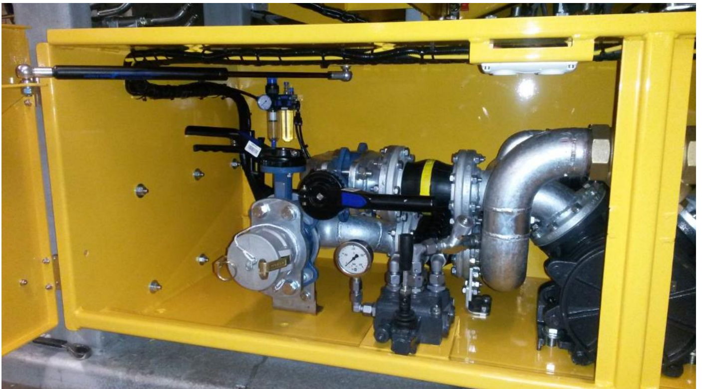
Detail: Left side of the cabinet with discharge outlet with 2 ½ inch cam-lock
