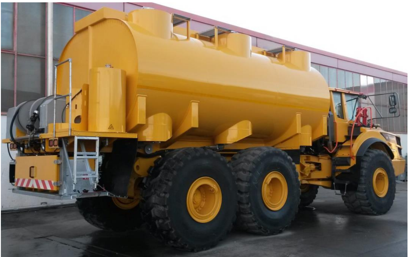
Rear right side view with coolant tank above the collapsible access ladder.
