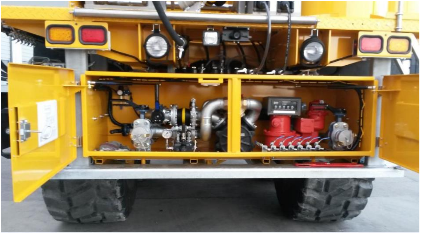
Steel cabinet at the rear side of the working platform mounted, with discharge outlets, with 2 ½ inch Cam-lock, pneumatic operations, pump and metering system. LED lights are mounted inside the cabinet which are operated by master-switch
