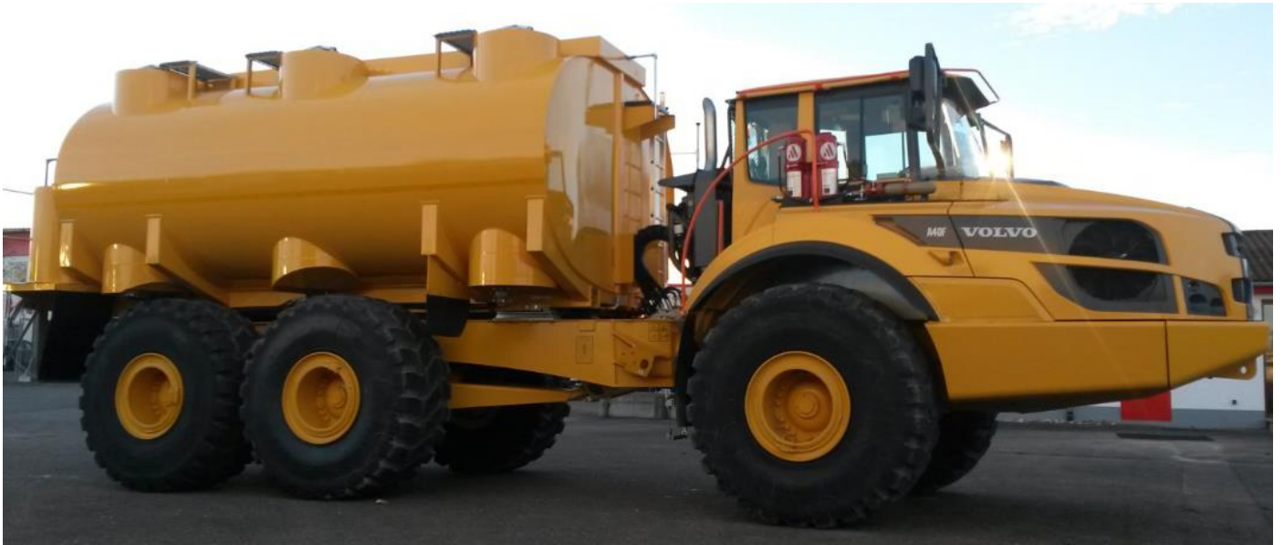
25000 ltr. tank for diesel fuel. / 4 x 1000 ltr. oil tanks / 1 x 1000 ltr. waste oil tank
