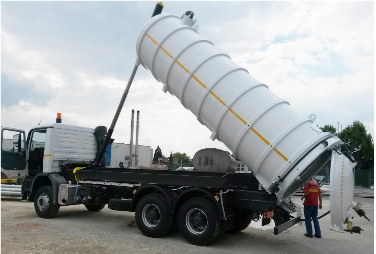
Vacuum Tank Version with Telescopic Tipping Cylinder (HYVA, Germany). Including Pneumatic Interlock System for additional safety.
