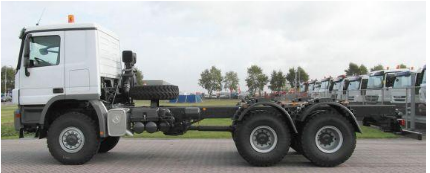
Truck chassis . Wheel base 4500 mm. M- or S-Cabin. 40 tons. Version (9/16/16 tons. axles)
