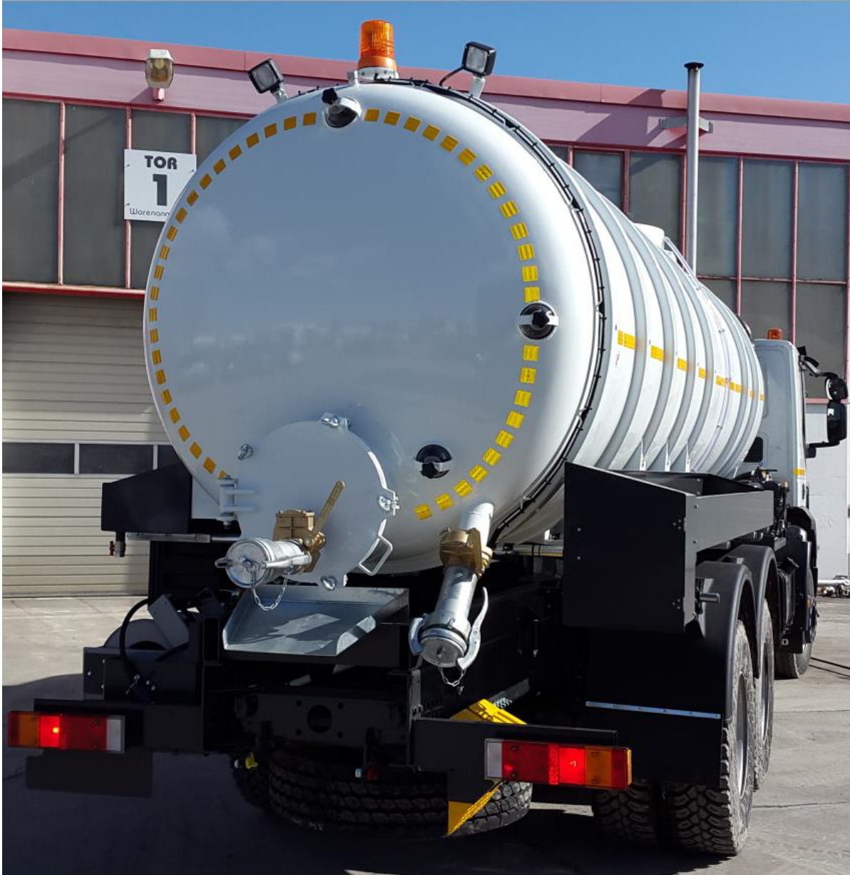
Vacuum Tank Version without hydraulic rear opening, but incl. manhole 600 mm. (Less cost)
