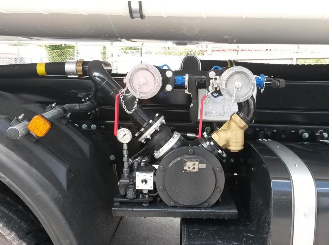
One self-sucking pump installed at the vehicle's chassis, hydraulically driven by PTO of truck engine. Pump made of stainless steel
