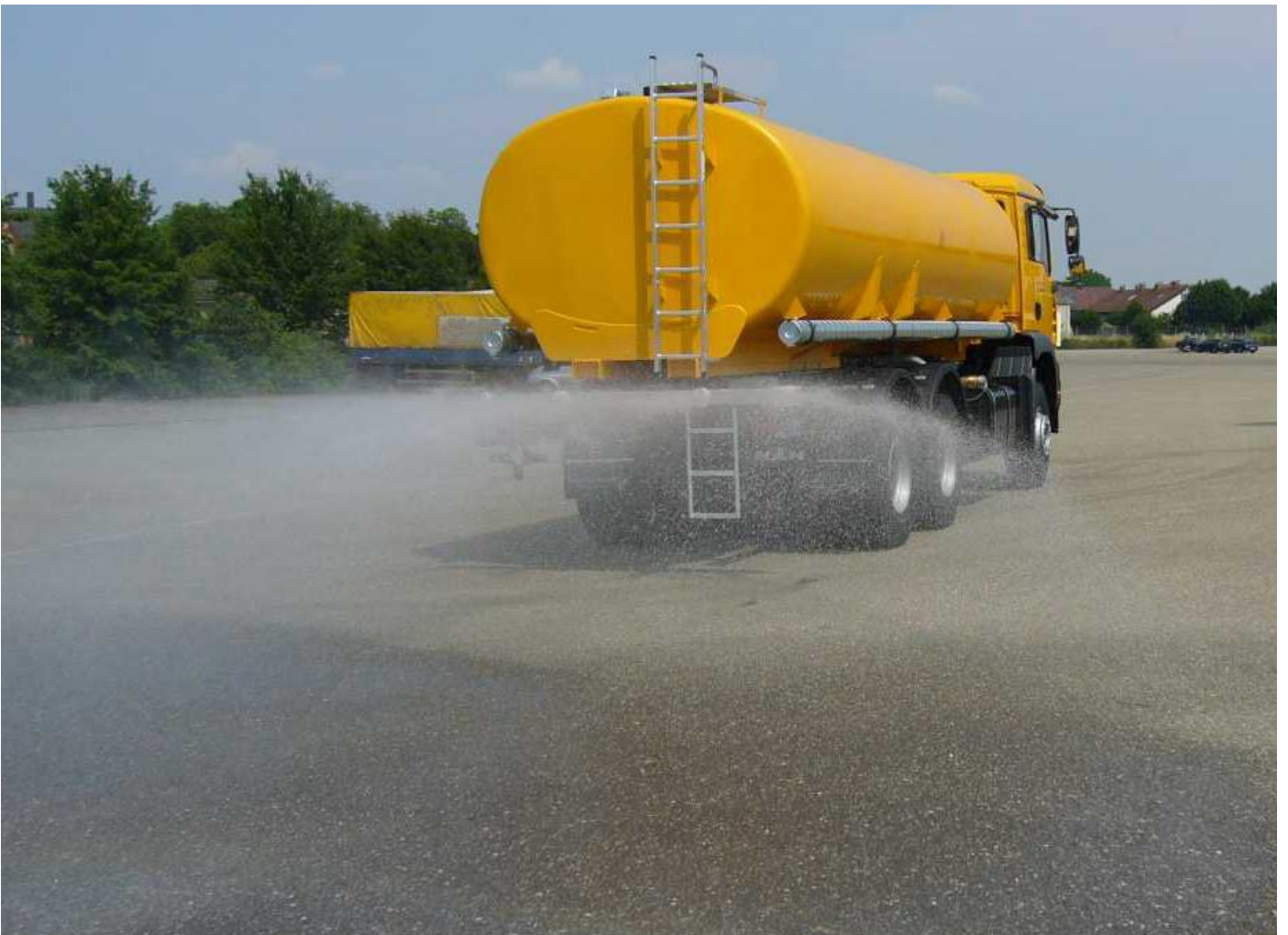
Operation of the spray bar out of driver's cab
