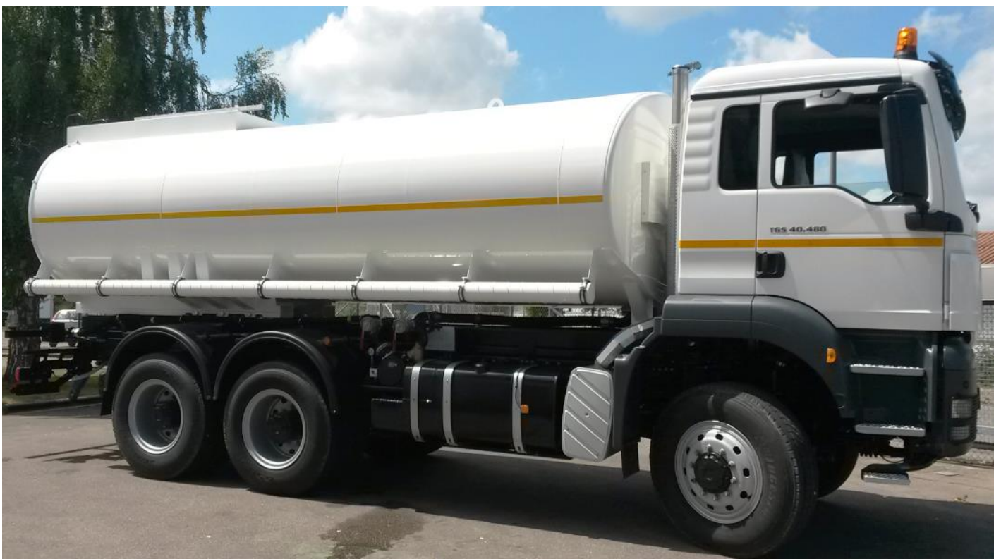
One hose-carrier on each side of the truck. The tank can be mounted on 6x4 and 6x6 truck chassis.
