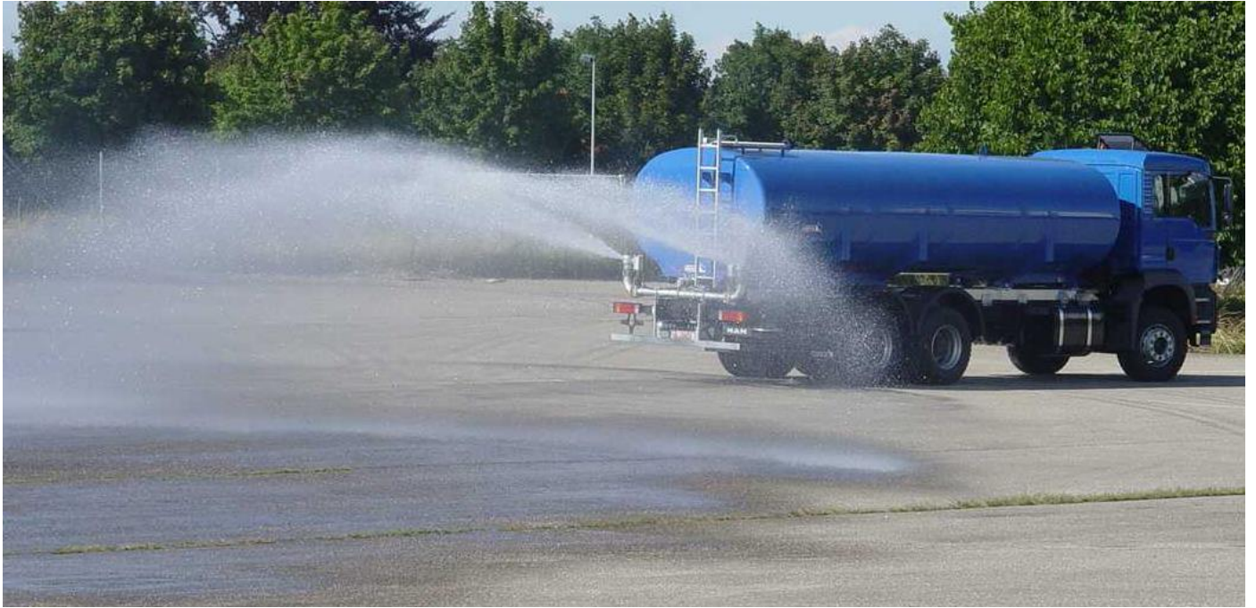
Spraying nozzle can be turned around by 360° Capacity: up to 400 ltr. / min each (adjustable)
