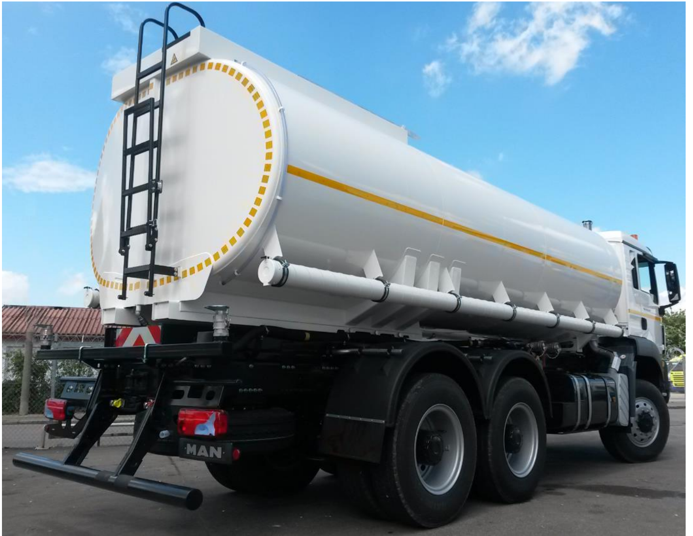
Access ladder and rear mounted spray bar with two special fan-nozzles (frog-type)
