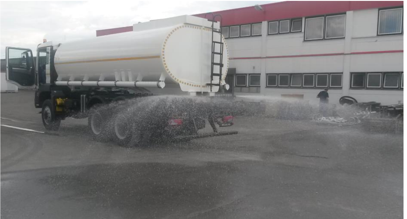
Some examples of the function of the adjustable spray bar mounted at the rear end of the tank truck
