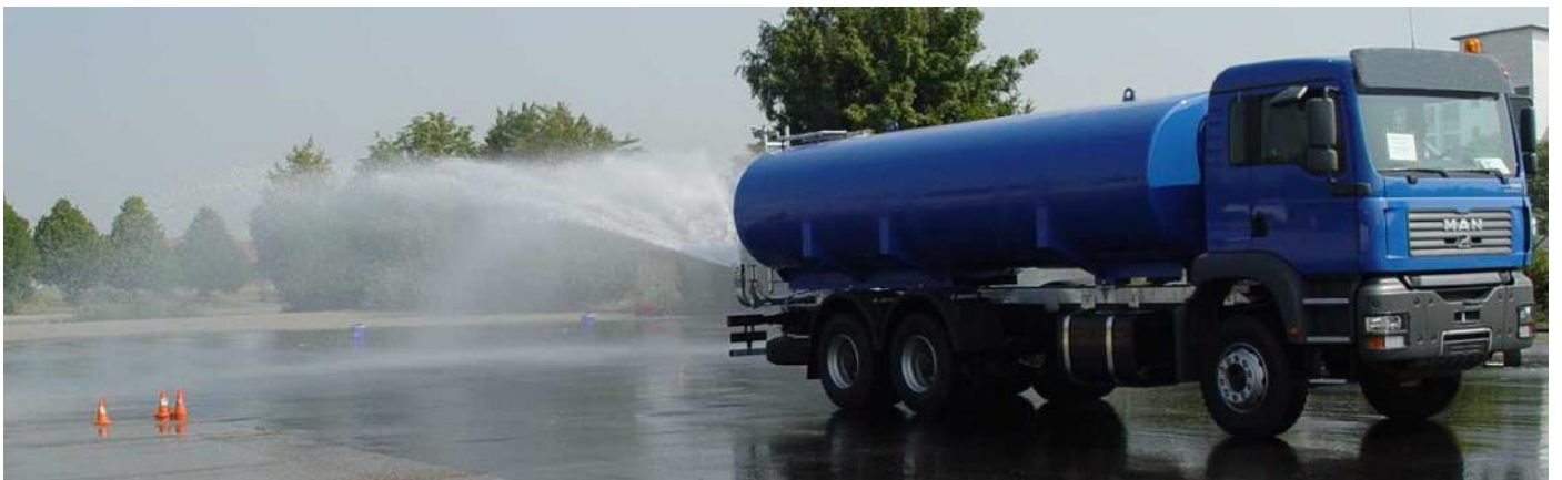
Spray bar rear: Adjustable spraying width with pump from approx. 10 to 12 mtr.
